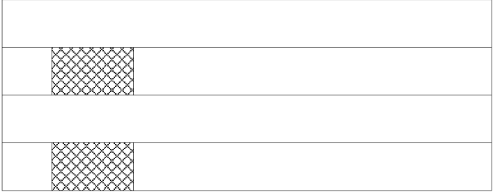
(c) 2-symbol short PUCCH can be transmitted in any two symbols within the configured PUCCH symbols
