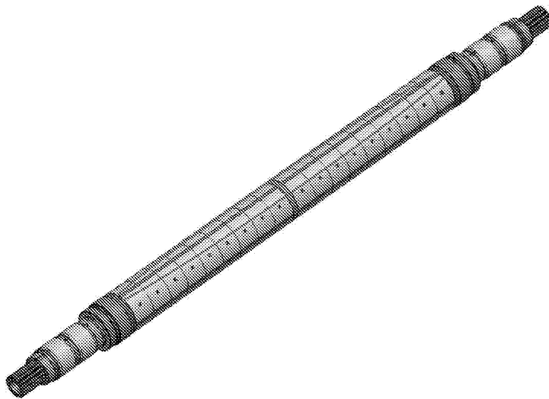
Figure 29 Rotor Shown without retention Sleeve – Notice dividing strip between magnetic poles
