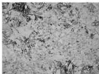
Comparative Example 7 (Forging Temperature 400 °C, \Delta \varepsilon = 3 )
