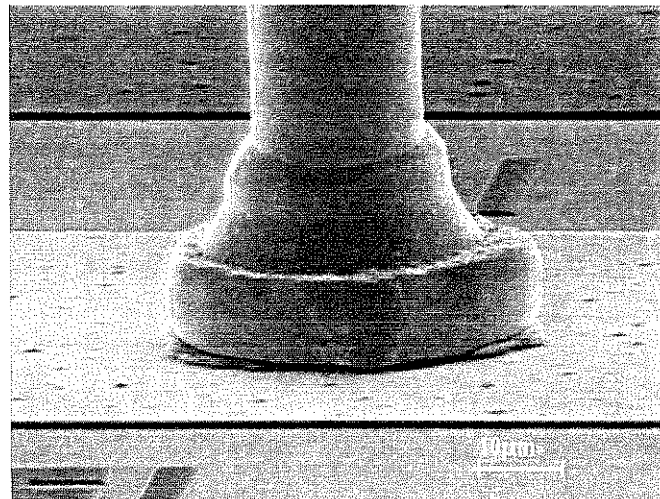
Fig 3(b) – Ball bond of 4N doped Cu 0.8mil wire
