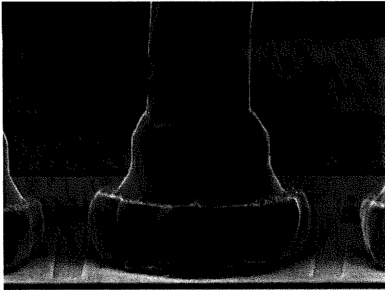
Fig 3 Ball bond of 3N Cu 0.8mil wire with trace additions
