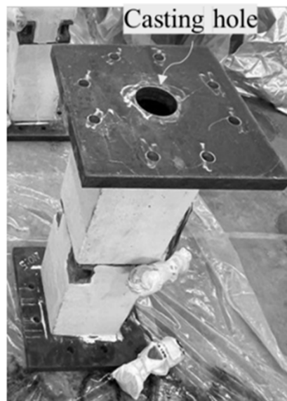
(c) Connection assembly
