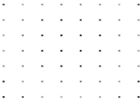
64QAM constellation diagram after a trade-off between communication performance and sensing performance
