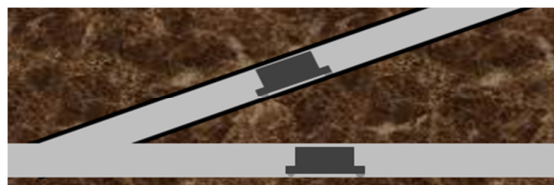
Fig. 7: access point with one bidirectional ramp
