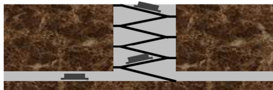
Fig. 5: access point with spiral road in shaft
