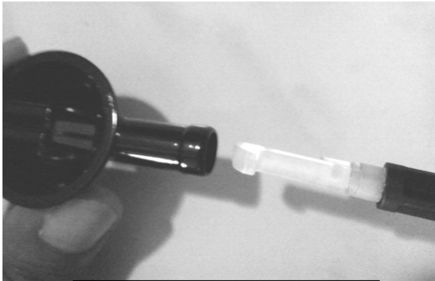
Figure 4: Attaching End of Target Stick
