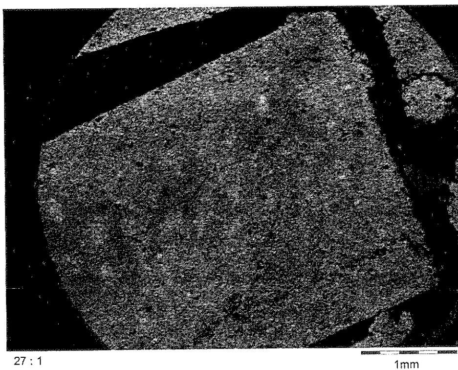
Fig. 8 b) EDX mapping of Cs
